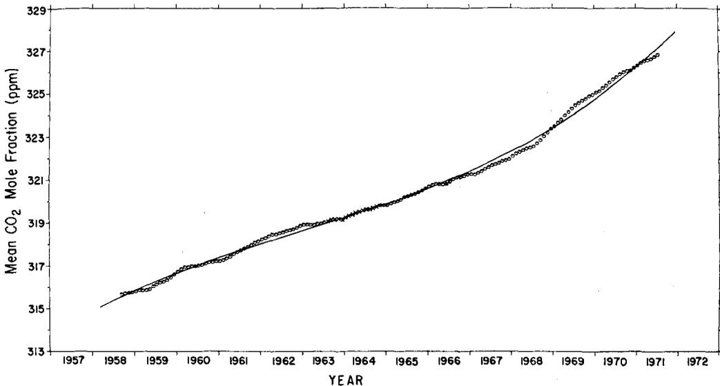
Fig. 9. Twelve month moving average of atmospheric CO<sub>2</sub> mole fraction at Mauna Loa Observatory. Circles: means plotted versus the seventh month of the appropriate 12 month interval. Crosses: means which include concentration estimates calculated from the oscillating power function for the period February, 1964 through May, 1964. Full curve: secular trend based on cubic trend function.
