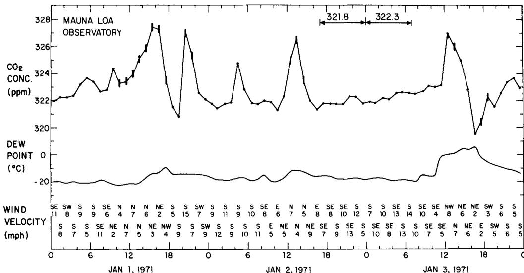
Fig. 1. Hourly average atmospheric CO<sub>2</sub> concentration at Mauna Loa Observatory versus time during the first three days of 1971. Concentrations are plotted on the adjusted CO<sub>2</sub> index scale. Vertical bars indicate periods during which the record trace was variable, indicating local contamination. Horizontal arrows indicate periods of steady concentration. The average concentration for each steady period is indicated above the arrow.
