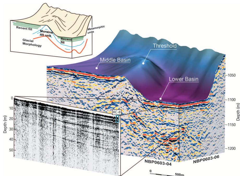
**Fig. 4. Three-dimensional view of seismic reflection data and multibeam bathymetry from Crane Fjord.** Seismic line locations are shown in Fig. 1, inset. Colored reflectors in block diagram are from Generator Injector Air Gun—seismic reflection, and the grayscale panel is from a 3.5 kHz compressed high-intensity radar pulse subbottom system. (Inset) Line drawing interpretation of layered and chaotic reflectors.
