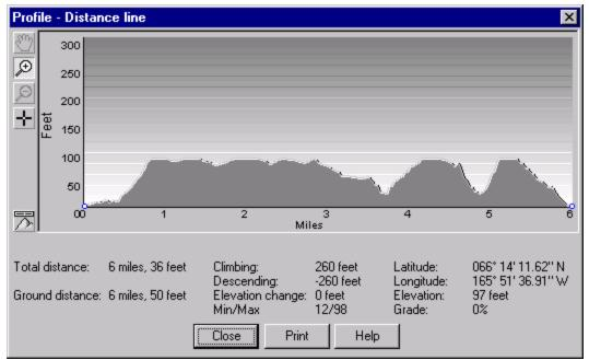
Figure 7 – East Nunatuq perimeter profile. The perimeter profile graphically shows the elevation differential around the boundary of the site investigated for the village.
